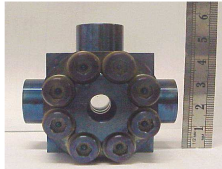
Fig. III: The HTI cell assembly. The cell itself is in the middle while the large screws are devoted to withstand high pressures (up to 500 bars) at high temperature (up to 600°C) [3].
