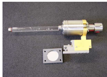
Fig. IV : the DSI cartridge. One can see on this picture the quartz cartridge containing the succinonitrile-camphor alloy (left), the compensator and motorization arm (right) [3].
